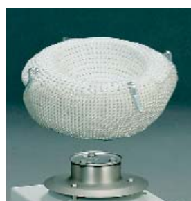
Stirring mantle with adapter device.
